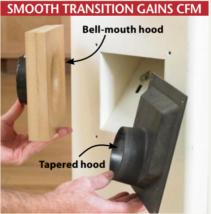
Adding either a bell-mouth hood or a tapered dust hood to any machine, such as this jointer, will increase dust removal.
