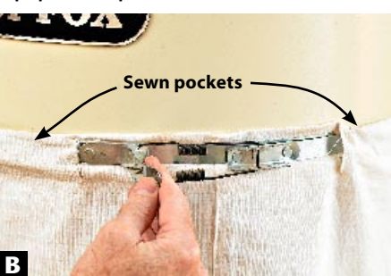
B Clamps in sewn pockets that open in only one spot prove easy to use.
