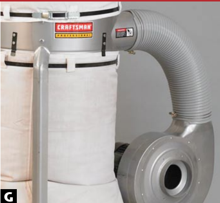
G The 6" hose on the Craftsman has a smooth transition from the impeller to the collection and filter bags.
