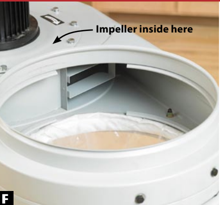
F The impeller on Delta's 50-760 blows dust and chips directly into the collection chamber without need for a jumper hose.
