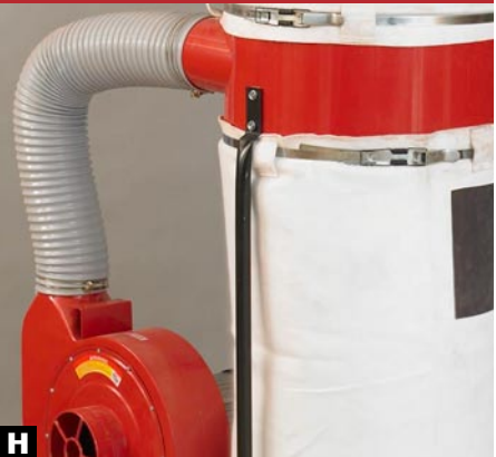
H The 5" hose on Penn State's DC2V2 bends at almost a 90° angle—creating more resistance—when the impeller is powered.
