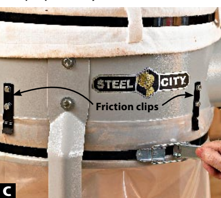
C Metal clips hold plastic bags while you secure the band clamp, which still takes two hands.
