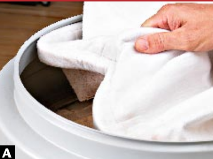
A Simply twist Delta's metal hoop slightly and it pops loose; put it back with a similar twist.
