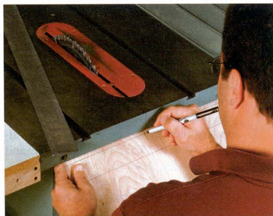
Transfer the mark. Slip the back plate under the top of the saw to transfer the center point of the arc from the saw to the plate.
