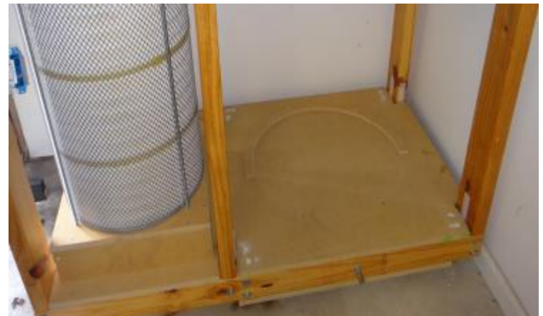
TRASH CAN BASE & FILTER – The base on the right is where the trash can sits. The half circle ring is used to position the trash can so it lines up with the separator. The filter is a Wynn Environmental (MERV15, pleated, open both ends) filter.
