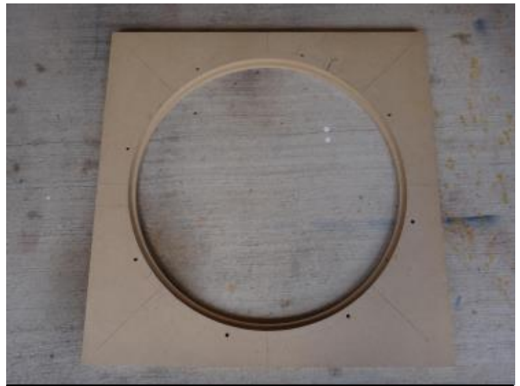
BOTTOM PLATE – Topside with the rabbet where the rubber weather strip will go to air seal the collector ring to the bottom plate. Holes are for the \frac{1}{4} " all thread rod.
