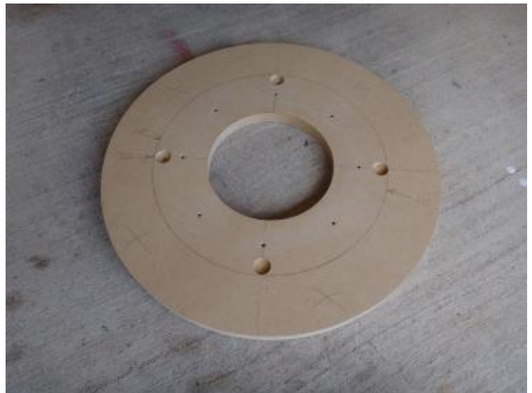
TOP COVER – Underside, recessed holes are for the nuts on the 1/4" all thread rod used to fasten the baffle to the filler ring.
