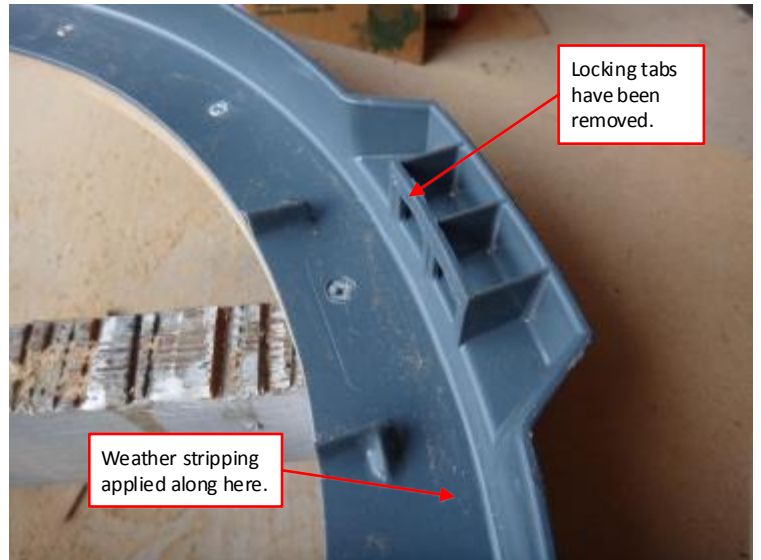
TRASH CAN RING – Locking tabs trimmed off handles so ring will not lock to trash can. Allows trash can to be freely lowered.
