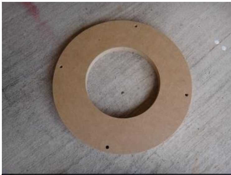
FILLER RING – Underside, holes are for the \frac{1}{4} " all thread rod used to fasten baffle to the filler ring. Outer diameter is slightly less than the inside diameter of the tapered cone inside collector ring.
