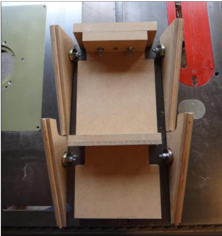
SLED – Partially exploded view showing sliding door rollers that will travel on \frac{1}{4} " dowels. \frac{1}{4} " dowels on ramps will be where rollers travel to raise base as sled moves forward. T-Nut captured in back between the two pieces of wood bolted together.
