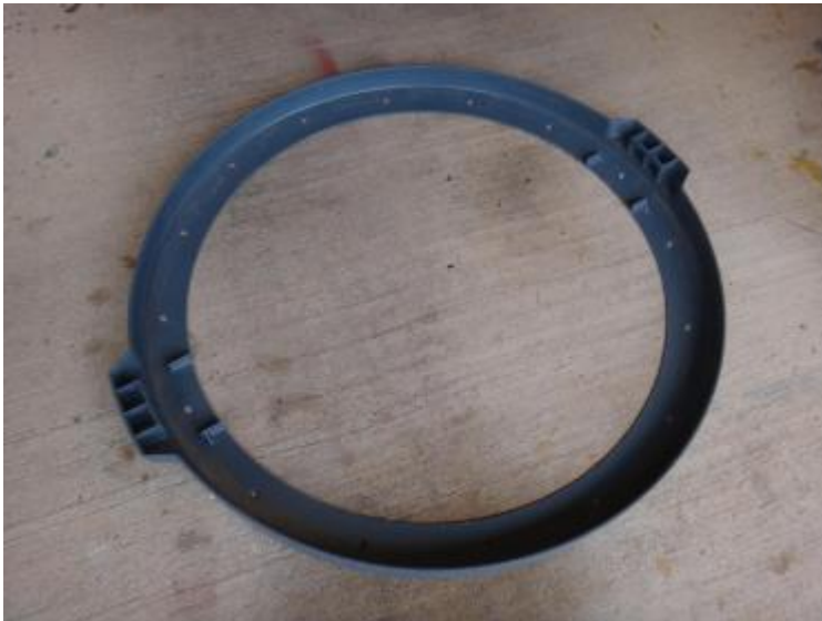
TRASH CAN RING – Trash can lid has been cut out to be flush with the bottom plate. Screw holes to fasten to bottom plate. Weather stripping will be added to provide air-tight seal to the trash can.
