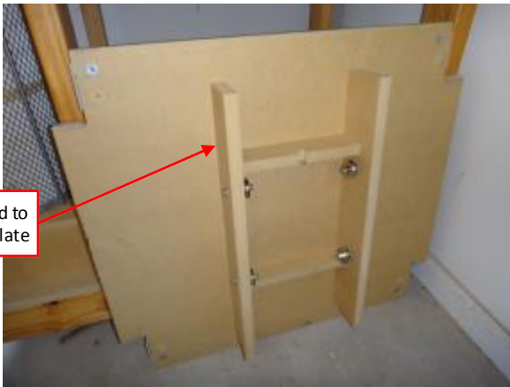
SLED – Partially exploded view showing sliding door rollers that will travel on \frac{1}{4} " dowels. \frac{1}{4} " dowels on ramps will be where rollers travel to raise base as sled moves forward. T-Nut captured in back between the two pieces of wood bolted together.
